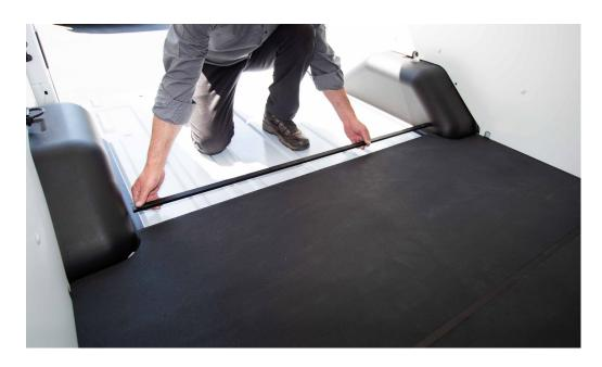
6. Attach the third floor piece (usually the largest) to the rail joint - use a rubber mallet so both floor pieces are secured tightly together.
