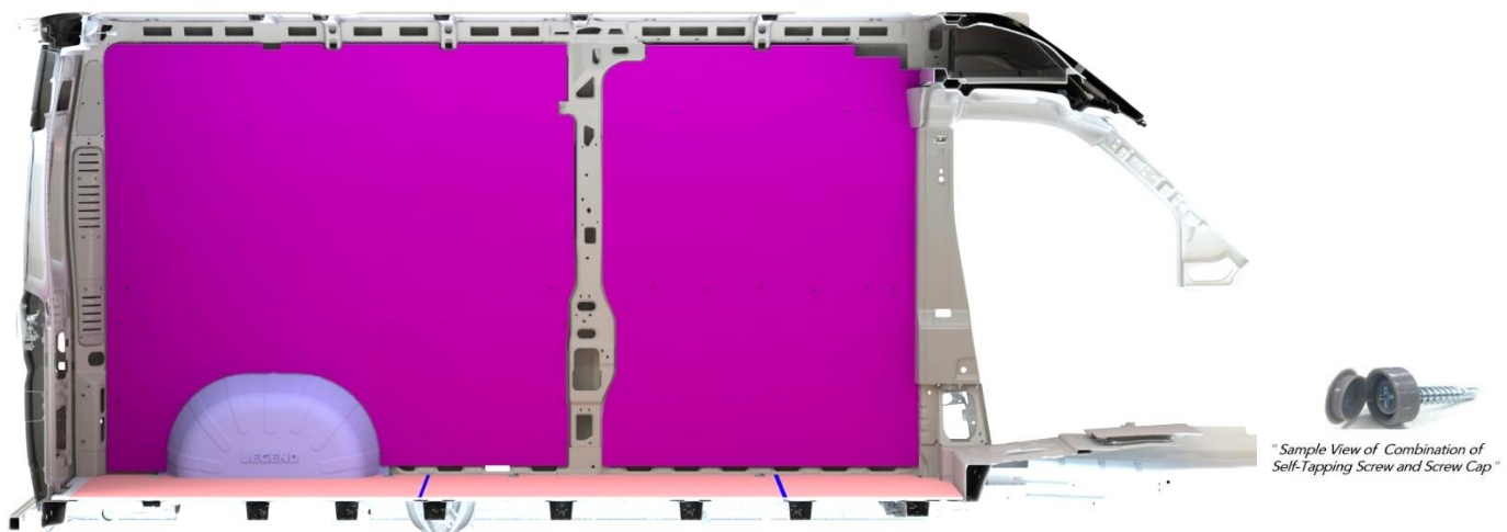
"Driver & Rear Side Front Wall Liner Installed" This is view from Inside of the Van- Viewing from Passenger Side
