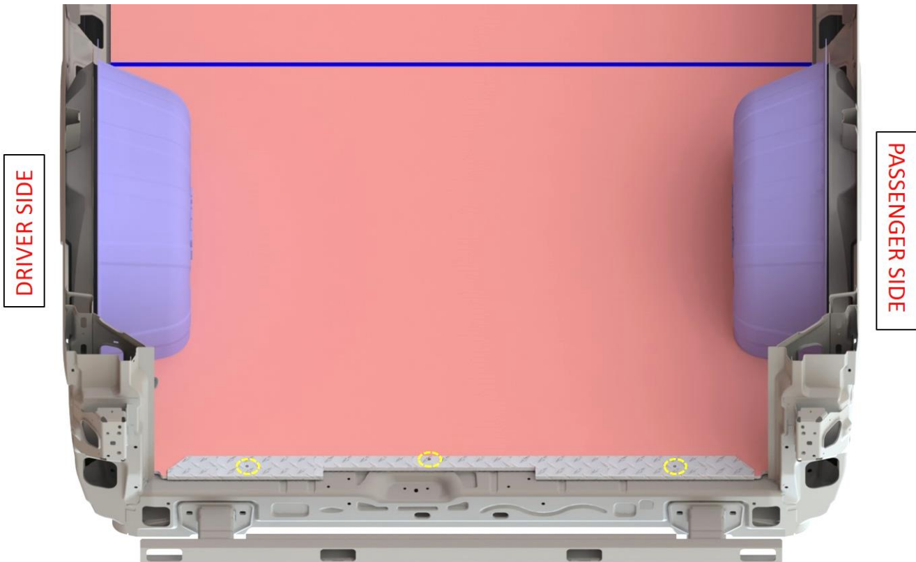
"Positioning and Fixing of the Rear Sill" This is view from Outside of Van- Viewing Towards Front
