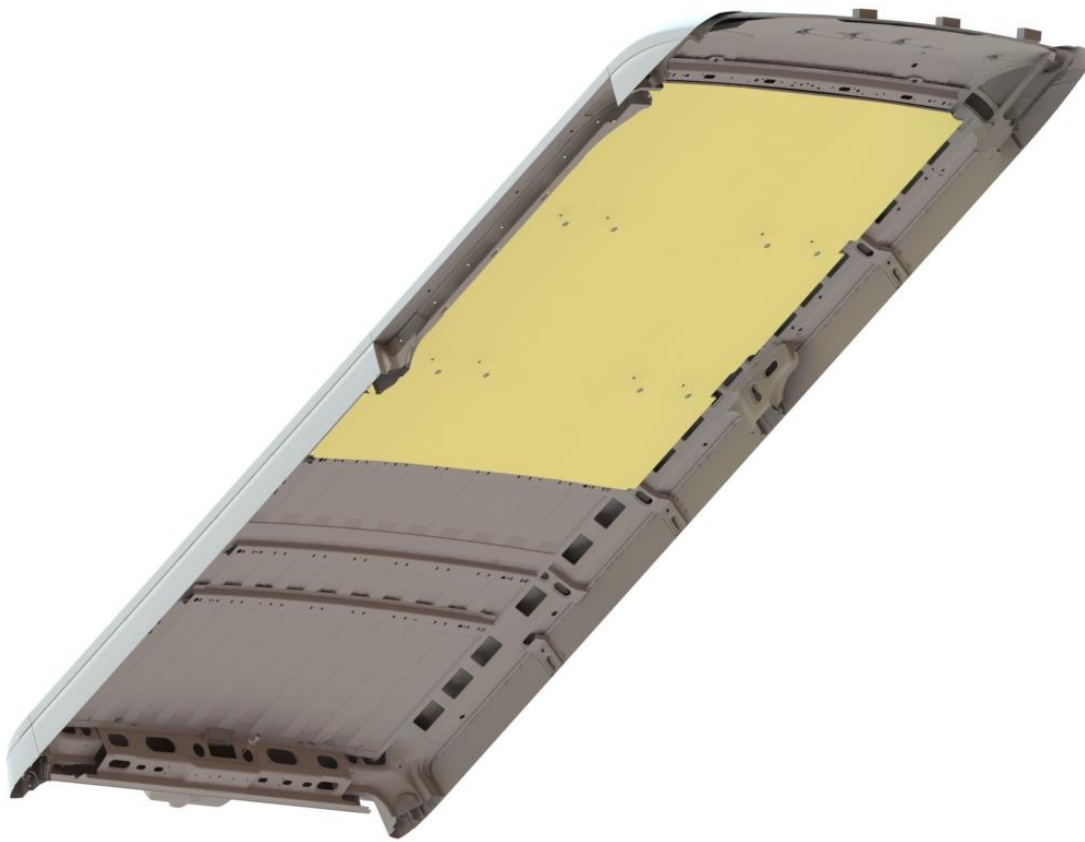
"Positioning and Fixing of the Front Ceiling Panel" This View is from Inside of the Van
