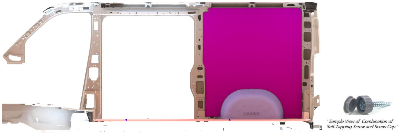
" Passenger Side Wall Liner Installed" (This is view from Inside of the Van- Viewing from Driver Side)
