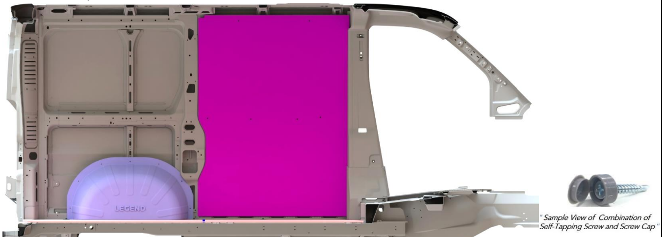
" Driver Side's Front Wall Liner Installed" This is view from Inside of the vehicle- Viewing from Passenger Side
