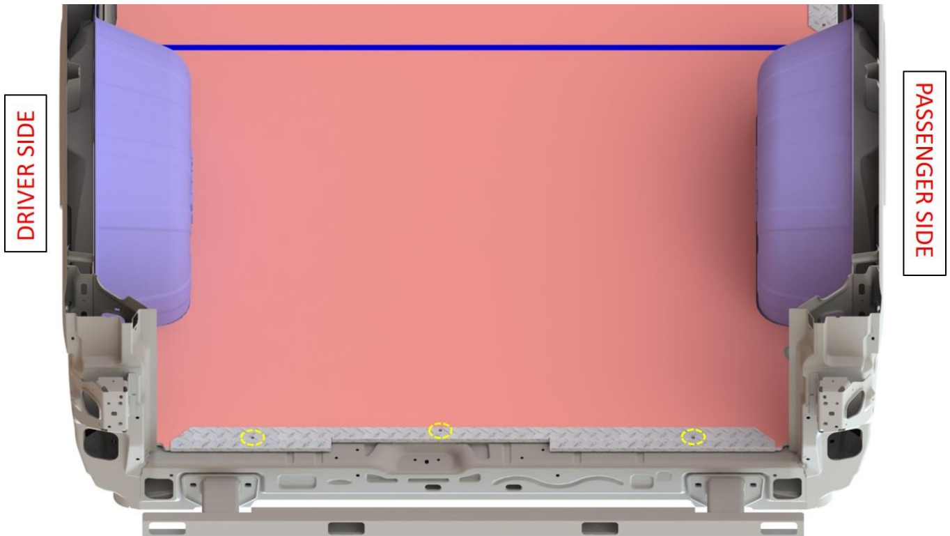
"Positioning and Fixing of the Rear Sill" This is view from Outside of Van- Viewing Towards Front
