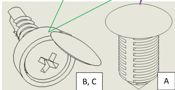
\*Note: Fix the right side of the panel with tape to keep it in position, make sure the tab on that edge is pushed inside the door cavity. With the tape holding the panel in position, pull the right side out, like a door, while holding it in position, install hardware (B,C) on the tab.
